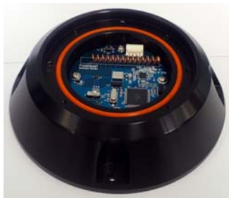
Fig. 2 The sensor node in enclosure (lid not shown)
