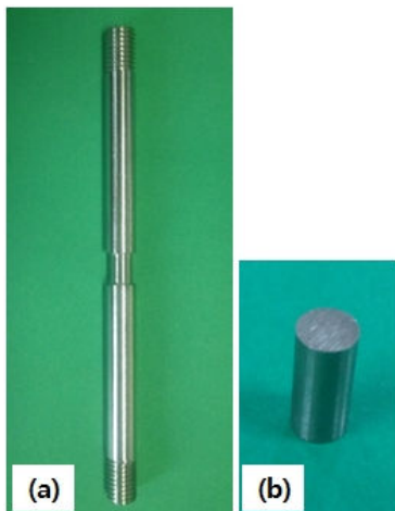
Fig. 2 Appearance of tensile (a) and compressive (b) specimen used in this study
