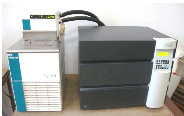
Fig. 3 Apparatus Holometrix 2300 for determination of thermal conductivity
