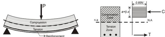
Fig. 1 Flexural Action of Reinforced Concrete Beam
