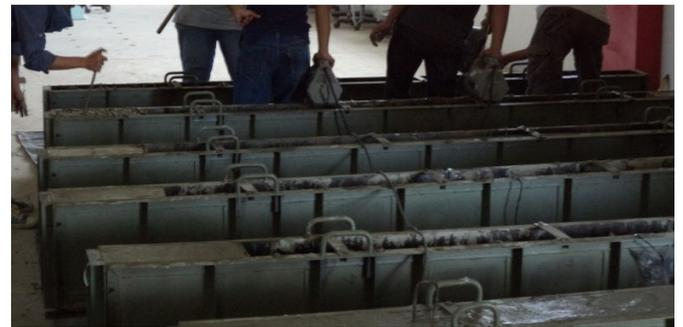
Fig. 3 Casting of Specimens
