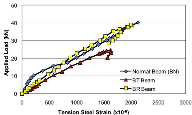
Fig. 8 Strain of the tensile reinforcement
