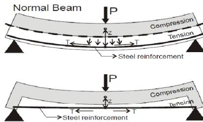
Fig. 5 Illustration of Flexural Action of Specimen BT
