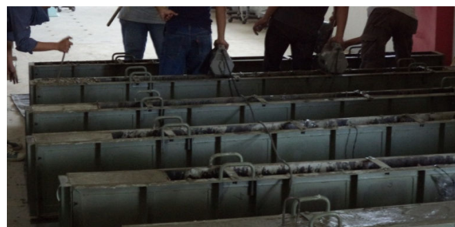
Fig. 3 Casting of Specimens
