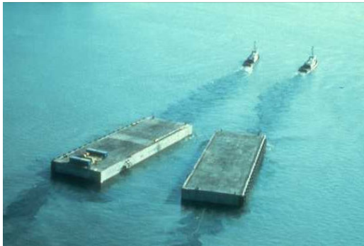
Fig. 3 Towing of pontoon modules [3]
