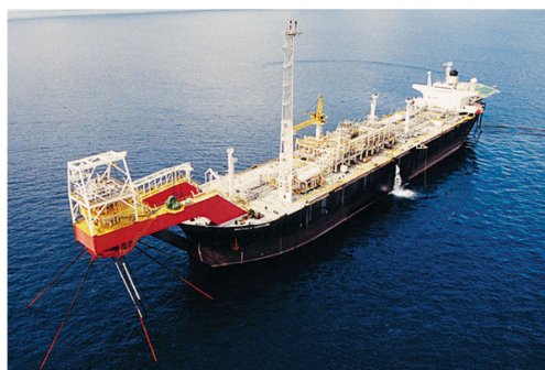
Fig. 1 Example of floating structure: FPSO [1]
