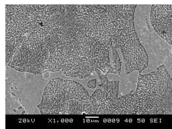
Fig. 3 (e) Microstructure of sample austenitized at 900°C and austempered at 325°C for 10 hours
