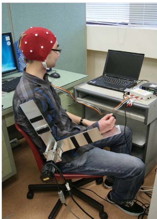
Fig. 2 A healthy subject to control the robotic arm by somatosensory stimulated BCI
