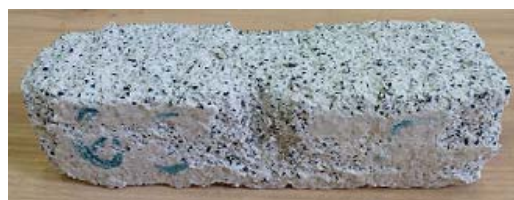
Fig. 10 PAG-10V specimen after 28 days of storing in SA solution
