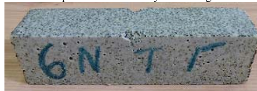
Fig. 11 PAG-10V specimen after 28 days of storing in NA solution
