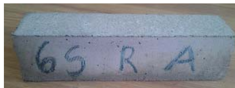
Fig. 8 PAG-10V specimen before the immersion in acid solution
