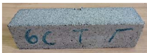
Fig. 9 PAG-10V specimen after 28 days of storing in CA solution
