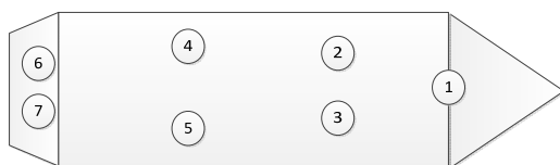
Fig. 3 The arrangement of thrusters
