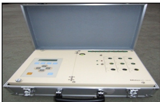
Fig. 6 Instrument of Microtremor GPL- 6A3P Model, Mitutoyo Corporation
