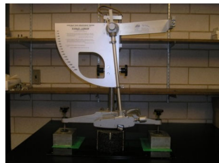
Fig. 4 Friction measurement setup using the BPT
