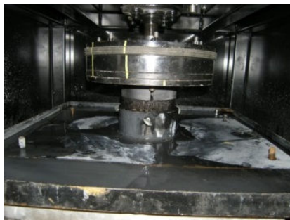
(b) Close-up of the rubber shoe-specimen interface
