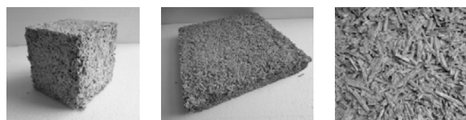
Fig. 2 The illustration of test specimens and the texture of filling materials
