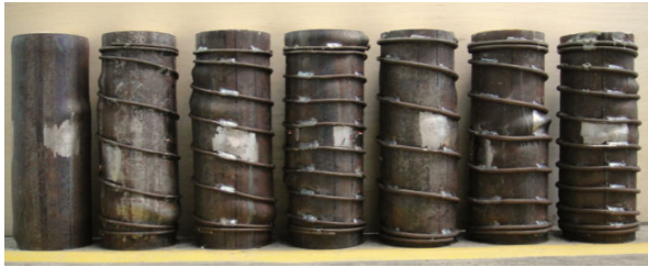
(a) Failure modes of confined HSCFST columns (100 MPa) From left to right: N0, S(6)20, S(6)15, S(6)10, S(8)20, S(8)15 and S(8)10
