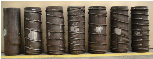
(b) Failure modes of confined UHSCFST columns (120 MPa) From left to right: N0, S(6)20, S(6)15, S(6)10, S(8)20, S(8)15 and S(8)10
