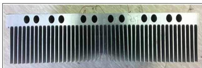
Fig. 6 Front view of the heat sink showing 12 flow holes in base
