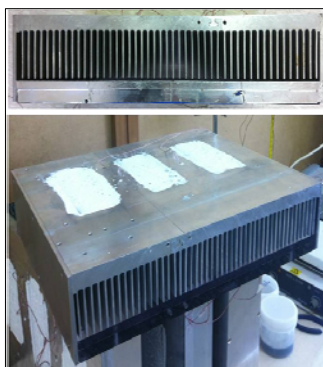
Fig. 2 Photos of the heat sink
