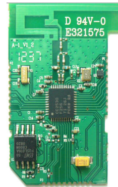
Fig. 2 Front of the processing and radio unit
