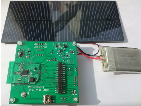
Fig. 4 Photo of the ZigBee sensor node with hybrid energy storage system
