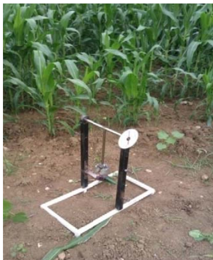
Fig. 1 Pendulum impact system
