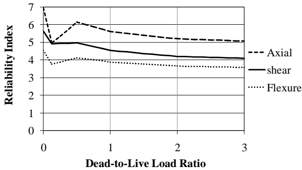
Fig. 1 Variation in reliability index with dead-to-live load ratio
