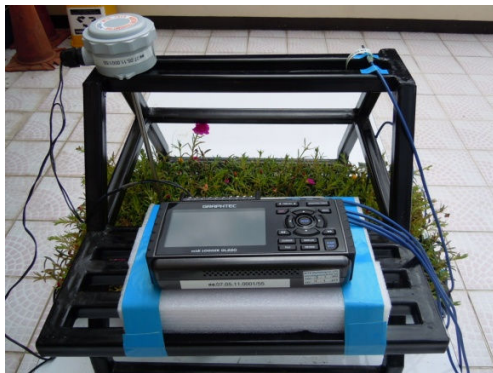
Fig. 8 The temperature measuring of purslane tray
