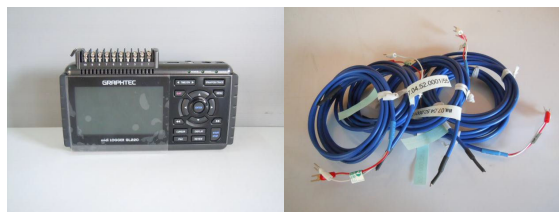
Fig. 4 Graphtec data loggers and thermocouple wires
