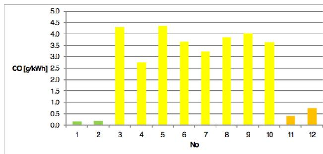
Fig. 6 CO emission for different helicopters engines
