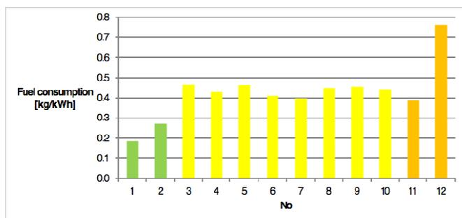
Fig. 4 Fuel Consumption for different helicopters engines
