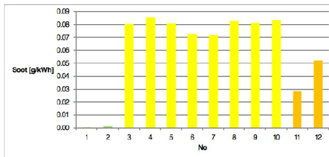
Fig. 7 Soot emission for different helicopters engines
