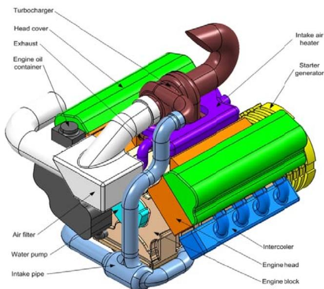
Fig. 2 Engine design
