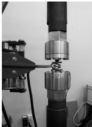
Fig. 2 Experimental apparatus for thermal fatigue test used in this study
