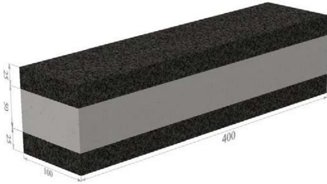
Fig. 13 Three-layer fiberconcrete (layers with fibers on the top and at the bottom)
