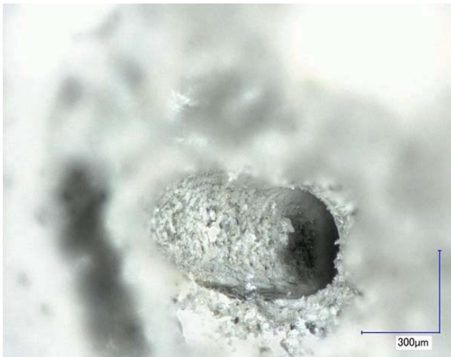
Fig. 10 Canal surface left by the orientated fiber at an angle of 80°
