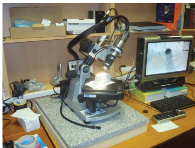
Fig. 1 Surface scanning at 40°
