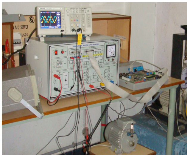
Fig. 16 Experimental setup of three-level inverter
