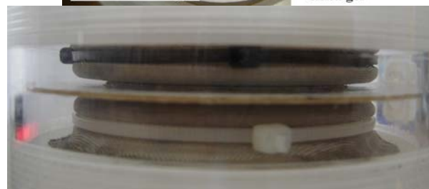
Fig. 5 Cardboard ring with silica gel balls
