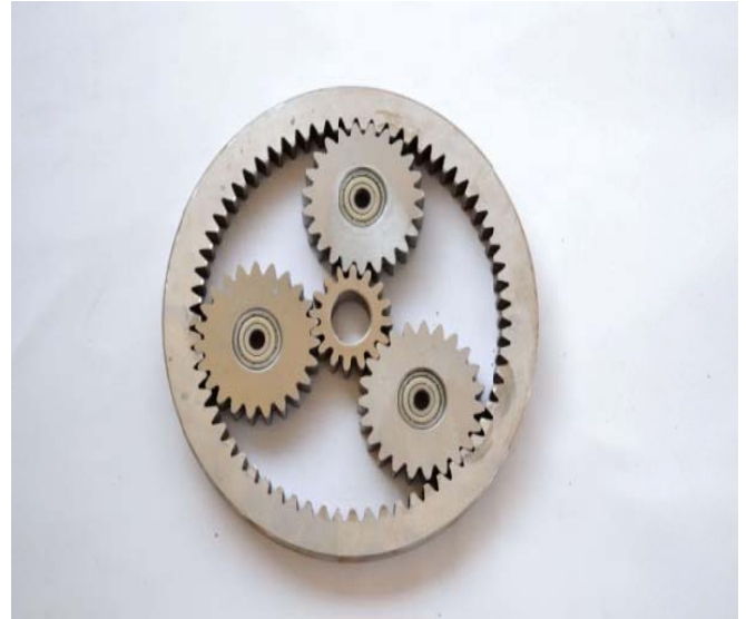
Fig. 4 Actual Manufactured Gears with bearings
