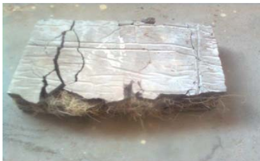
Fig. 5 Sisal fibre reinforced tested slab (3% fibre)
