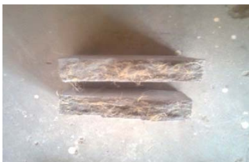
Fig. 4 Sisal fibre reinforced tested slabs (1% fibre)
