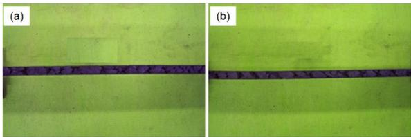
Fig. 2 Appearances of the ingots (a) S0 and (b) S1 after hot rolling
