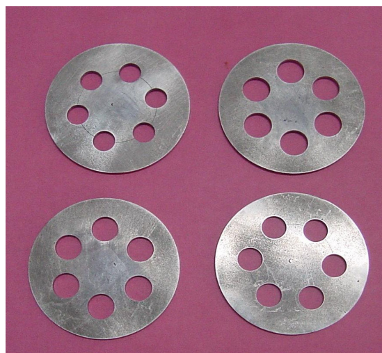
Fig. 10 Orifice plates for blanket zone (Typical)
