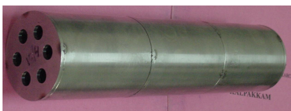
Fig. 11 Orifice assembly for blanket zone (Typical)
