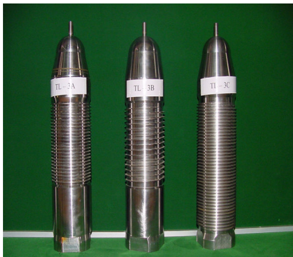
Fig. 15 Top labyrinths for model testing
