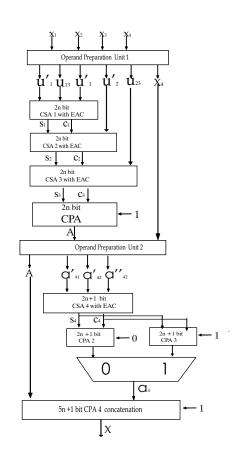
Fig. 1. Proposed hardware Structure
