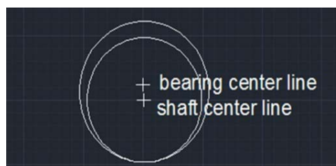
Fig. 1 Bearing center line and shaft center line position in shaft sleep condition
