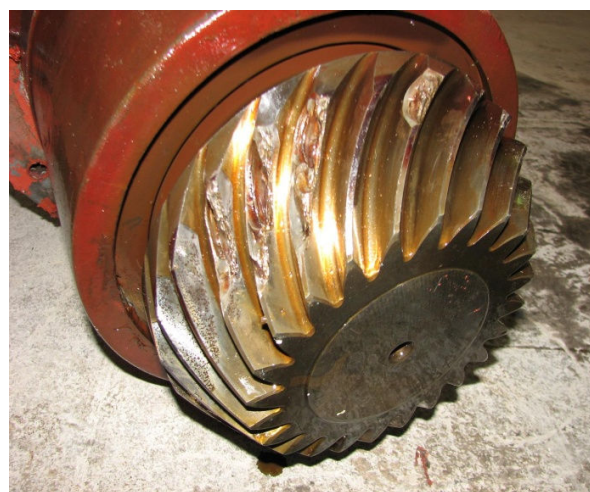
Fig. 16 Damaged gear (pinion)
