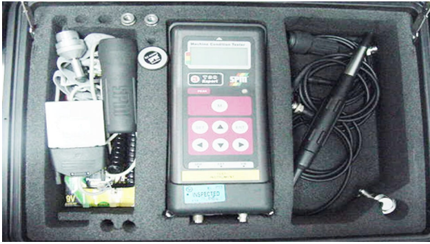
Fig. 2 Shock Pulse Transducer with Probe TRA-22 and a typical SPM data collector
