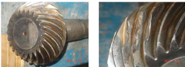
Fig. 18 Damage in gears in the next stage
