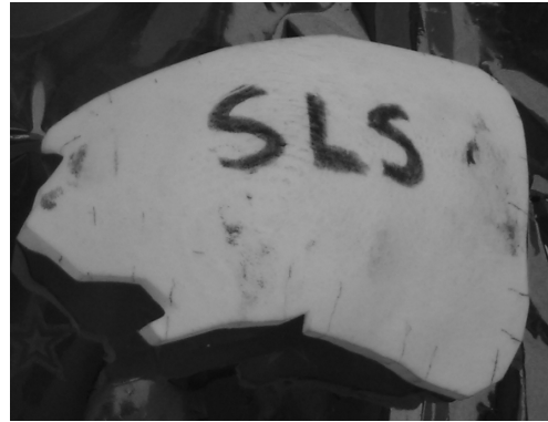
Fig. 9 Physical model of the cranial defect produced using SLS RP machine
