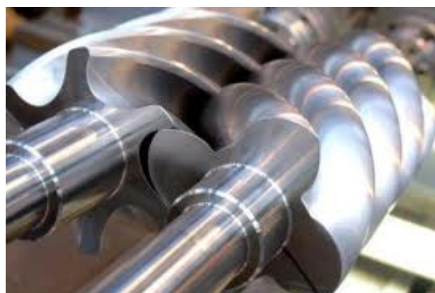
Fig. 1 Typical twin rotary screw compressor main rotor clearances down and basic operation principals up
