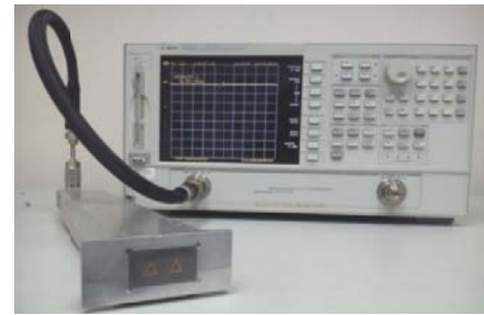
Fig. 5 Scattering parameters measurements setup
