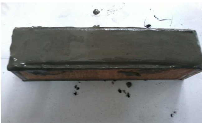
Fig. 2 CNT/Cement mixture in wooden mould
