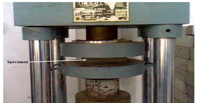
Fig. 4 Hydraulic Mechanical Testing System
