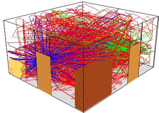
Fig. 3 Visible rays received by receiver inside room
