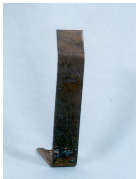
Fig. 6 The photograph of a test electrode copper of 1mm thickness
