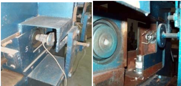
Fig. 7 Load cells attached with the roller bearings
