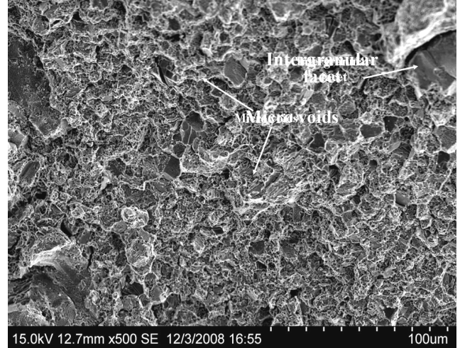
Fig. 8 Fractured image of the 21-4N SCT specimen
