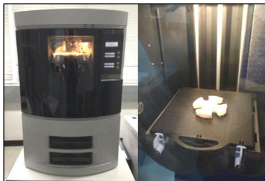
Fig. 23 RP machine-FDM Process
