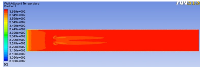
Fig. 13 Contours of wall adjacent temperature at Re 1200
