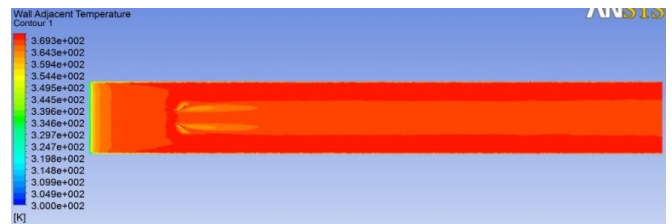
Fig. 15 Contours of wall adjacent temperature at Re 2000
