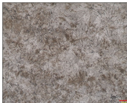
Fig. 1 The initial microstructure of SK85 high carbon steel used in this study
