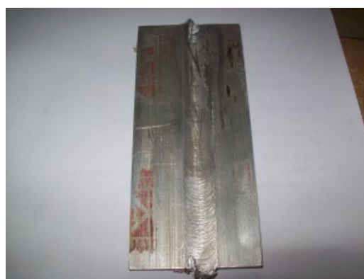
Fig. 11 Friction stir welded aluminum alloy H20 triangular tool
