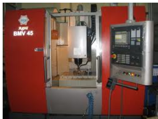
Fig. 2 CNC milling machine BMV 45
