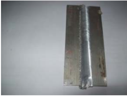
Fig. 12 Friction stir welded aluminum alloy H20 taper cylindrical tool
