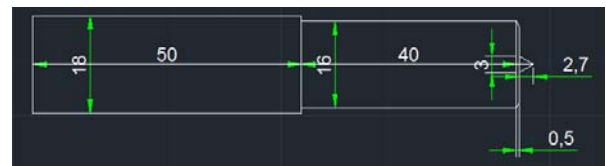
Fig. 7 Friction stir welding triangular tool
