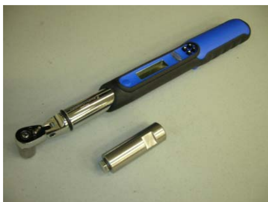
Fig. 8 Torque Wrench and Adapter Tool
