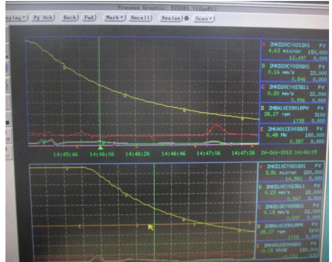
Fig. 10 Shutdown vibration of generator journal after balancing process
