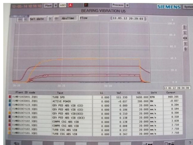
Fig. 2 Vibration condition in first balancing stage
