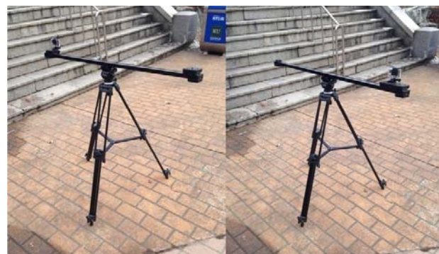
Fig. 2 Stereo video acquisition using Gopro
