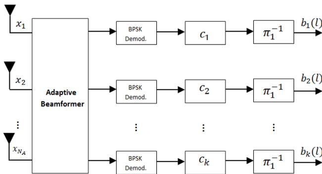
Fig. 3 CI-CDMA Receiver with antenna array
