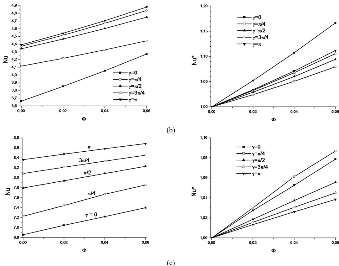
Fig. 16 Variation of the average Nusselt number and dimensionless average Nusselt number as function of solid volume fraction for different phase deviations for  $Ha=0$ ,  $Ra=10^3$  (a)  $Ra=10^4$  (b) and  $Ra=10^5$  (c)
