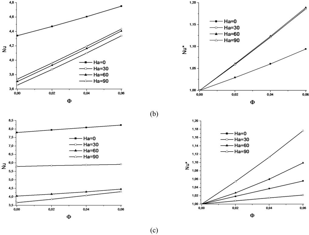
Fig. 11 Variation of the average Nusselt number and dimensionless average Nusselt number as function of solid volume fraction for different Hartmann number for  $\gamma=\pi/2$ ,  $Ra=10^3$  (a)  $Ra=10^4$  (b) and  $Ra=10^5$  (c)
