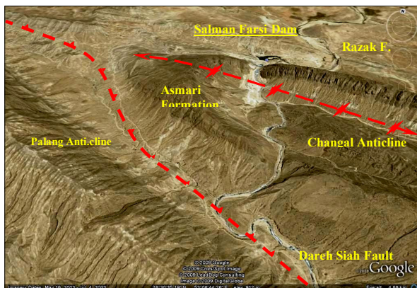
Fig. 2 Satellite image of Salman Farsi dam project constructing on the northern flank of Chngal Anticline at the Zagros folded belt
