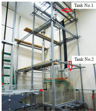
Fig. 9 Picture of Tanks No. 1 and 2 in the water supply cycle (MFL-TMU)
