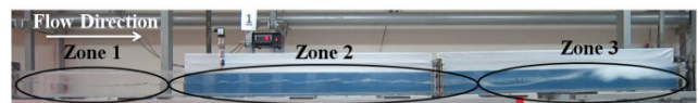
Fig. 2 Three regions of slug flow, \alpha_l=0.75 , U_{sl}=0.22 m/s and U_{sg}=5.09 m/s, Tarbiat Modares University Multiphase Flow Lab. (MFL-TMU), Test No. 6
