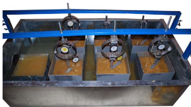
Fig. 1 Saturation-Drying Tank for Piles Uplift Pressure
